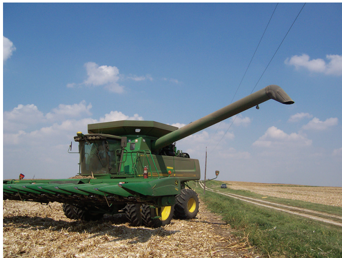
Use care when raising augers or the bed of grain trucks around power lines.
